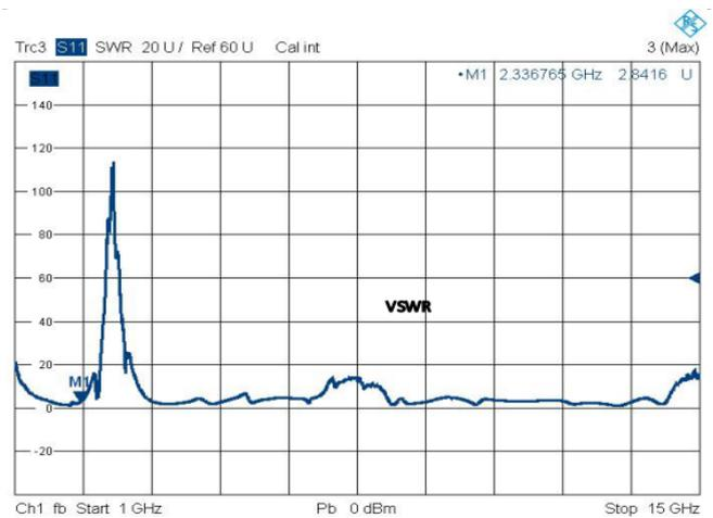
Fig.14. The measured VSWR of the proposed antenna
