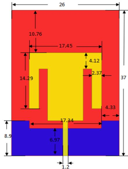
Fig. 5. Geometry of the proposed antenna structure.
