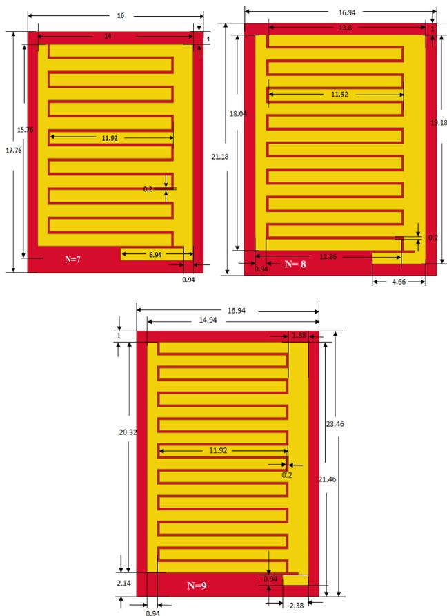
Fig. 1. The proposed CRLH-TL unit cells structure for  $N=7, 8$  and 9 fingers.
