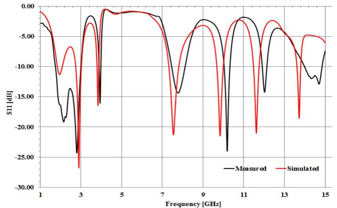
Fig. 9. Simulated and measured reflection coefficient of proposed tri-band antenna.
