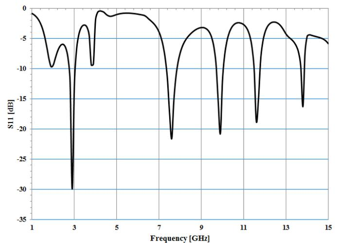
Fig. 2. The simulated  $S_{11}$  [dB] of the proposed DGS antenna.
