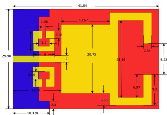
Fig. 1. Geometry of the proposed antenna structure.
