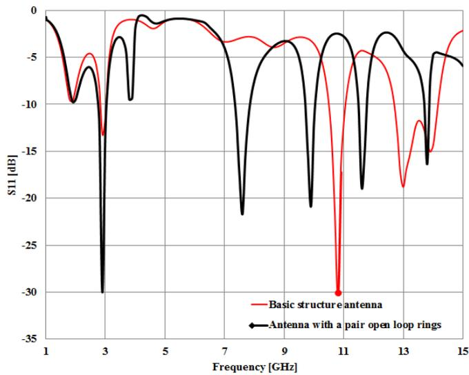
Fig. 4. Simulated reflection coefficient of various antenna designs.
